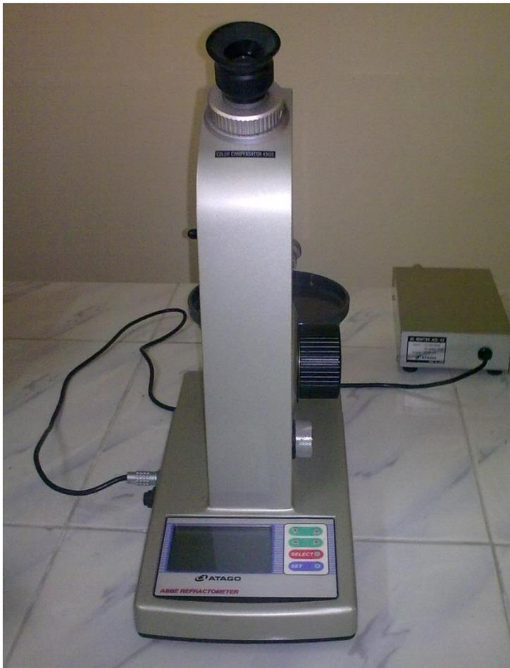
Used For the determination of refractive index, Total Soluble Solid (TSS) of oil, water, fruit juice, milk etc.
