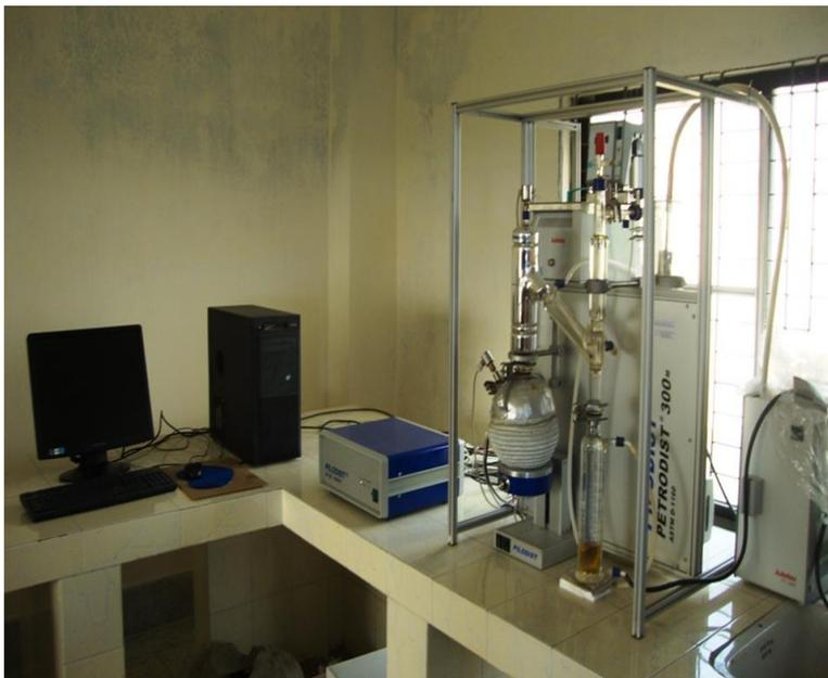
Used for the separation of pure organic solvents, hydrocarbons from the crude substituents.
