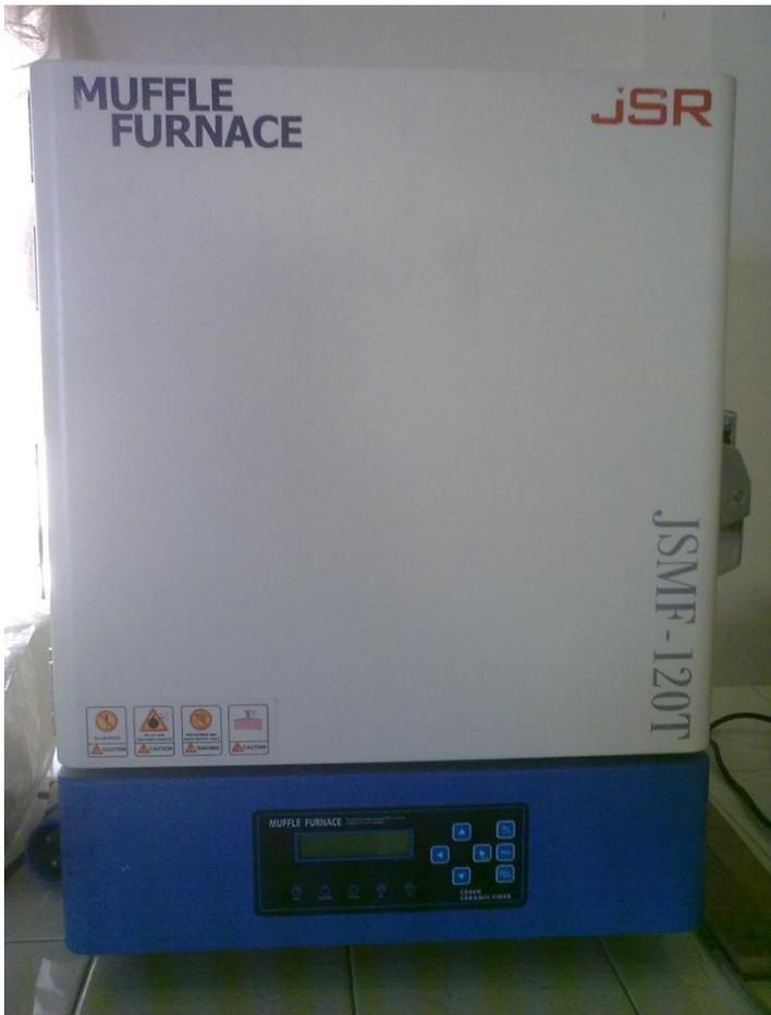
Used For: Materials heating at controlled programmable temperature up to 1200°C
