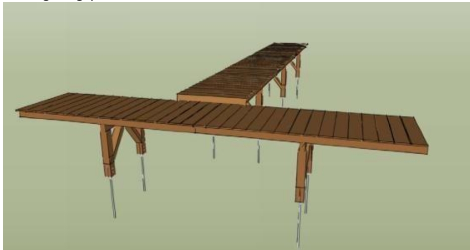
Figure 47: Isometric view of Jetty looking towards mainland
