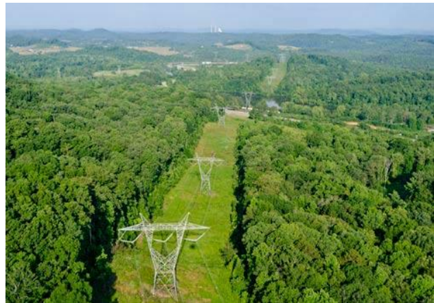
Figure 41: Fig: Right of Way (RoW)
