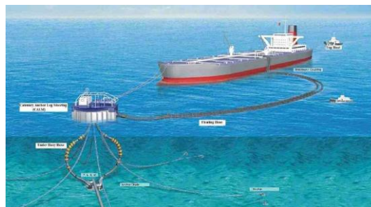
Figure 12: Single Point Mooring (SPM) with Double Pipeline
