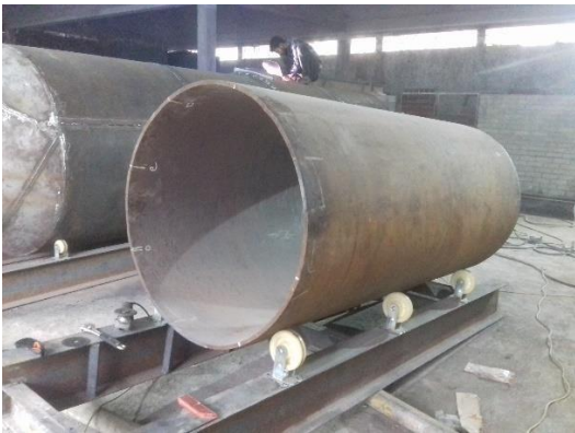
Figure: Ball mill under fabrication
