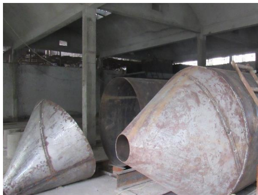
Figure: Silo under fabrication
