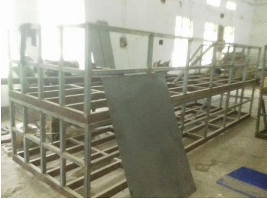
Figure: autoclave mold under fabrication
