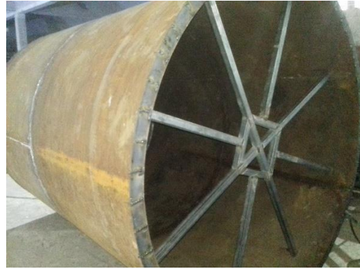
Figure: slurry tank under fabrication
