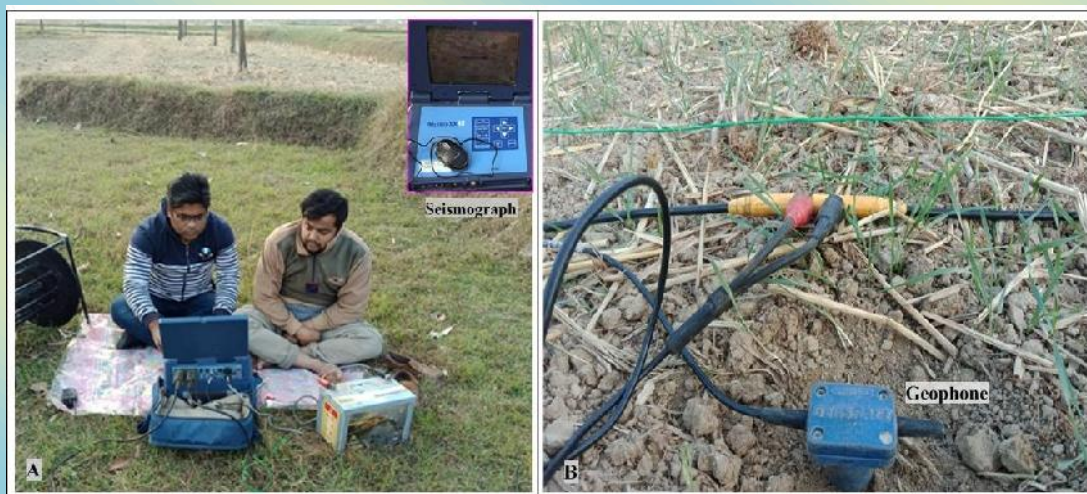
Figure-2: Seismic data recording unit (A) Seismograph and (B) Geophones with multi-core cable.
