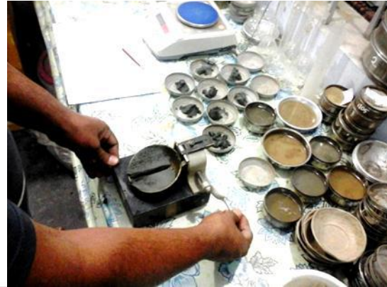
FIG-5. Atterberg Limits test in Progress
