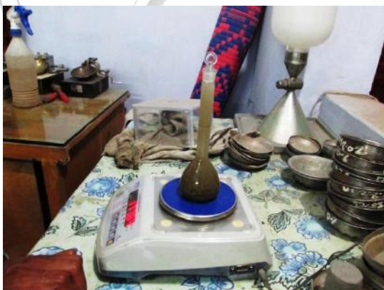
FIG-8. Specific Gravity test in Progress
