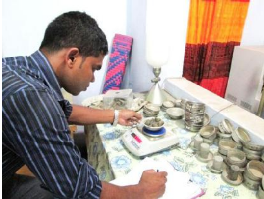
FIG-4. Moisture Content test in Progress
