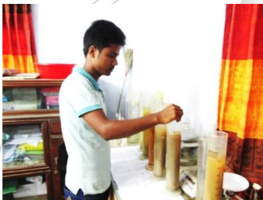
FIG-6. Grain size analysis (Hydrometer) test in Progress
