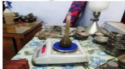
Specific Gravity test in Progress
