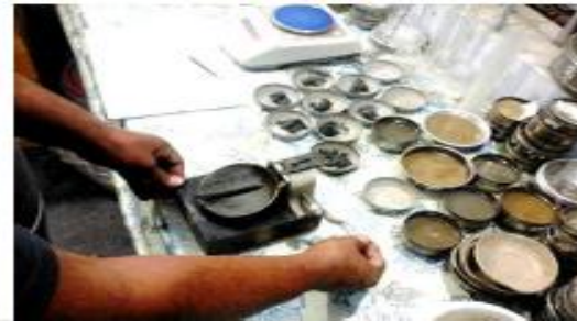
Atterberg Limits test in Progress
