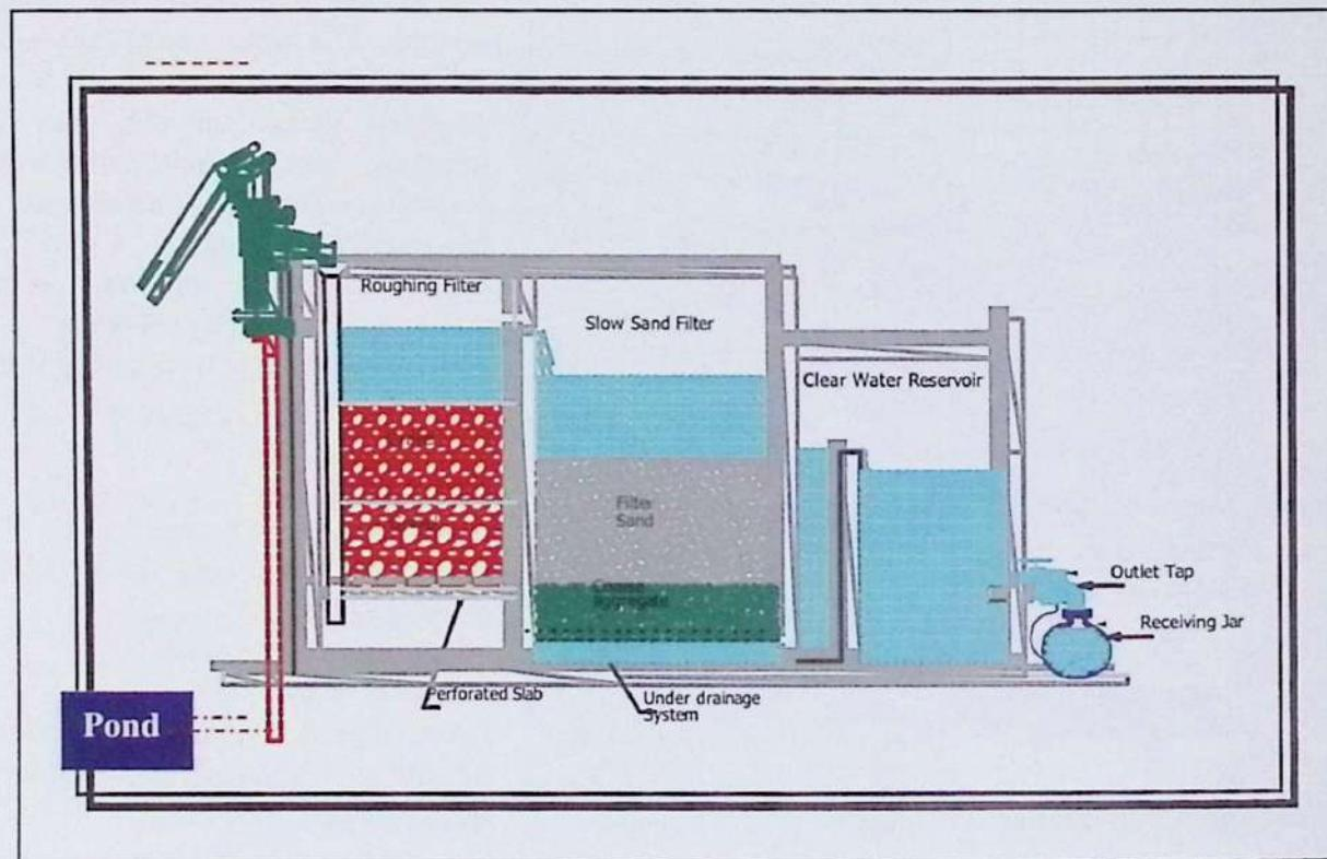
Raw water from pond is pumped up from a pond; the turbidity gets down through the roughing filter and then discharged into the filtration unit. The water is filtered and then collected in a clear water reservoir by an under drainage system. PSF is a good option for arsenic mitigation as well as for salinity prone areas
