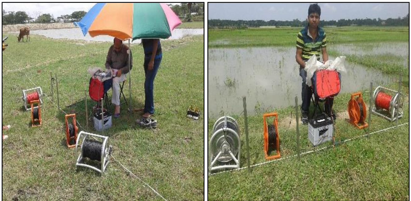
Figure 13: Survey required instruments (Resistivity meter, Battery, Cable reels)
