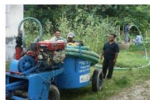
Vacutug Mark II Capacity: 120 Liters/Min
