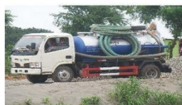
Vacutug with a capacity of 2000 Liters
