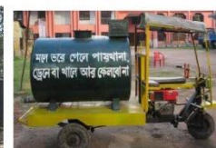
Mechanized Transporter (Mounted on Tri-Wheeler Diesel Engine Driven Vehicle); Capacity: 1300 Liters
