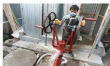
Mechanized Gulper Capacity: 60 Liters/min
