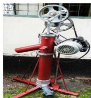
Motorized Gulper Capacity: 90 Liters/min
