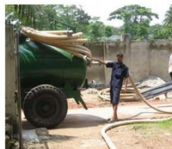
Sludge collection from septic tank with vagutug at Lakshmipur Pourashava
