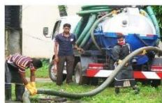
Vacutug Mounted on Pickup Capacity: 250 Liters/Min
