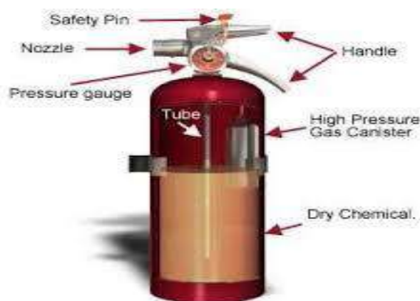
Fig 7.1: Different parts of Portable Extinguisher
