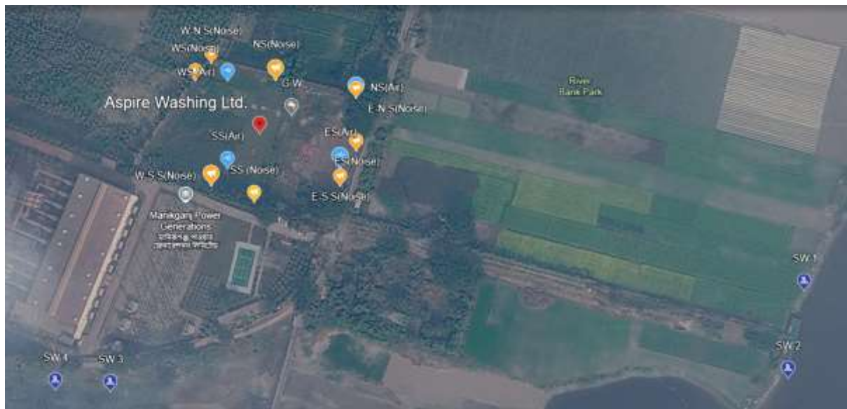
Figure 4.3: Location of Environmental Monitoring Samplings of Aspire Washing Ltd.
