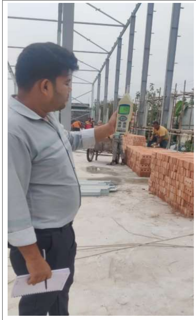
Figure 4.14: Ambient Noise Measurement
