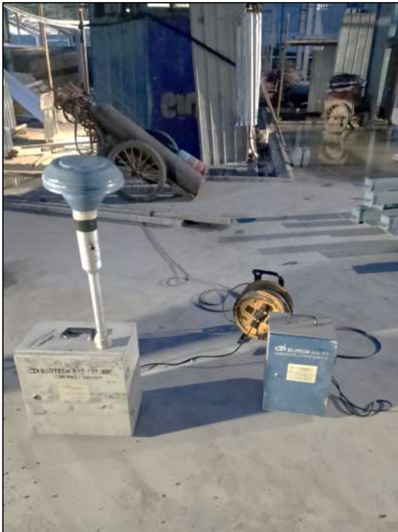
Figure 4.11: Gravimetric Sample Collector for Ambient Air Quality Measurement
