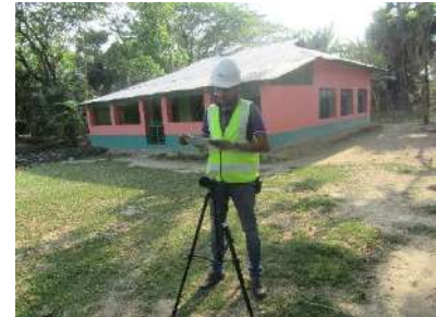
Noise measurement in the field
