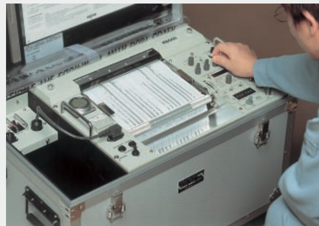
Recording the echo of a drilled hole
