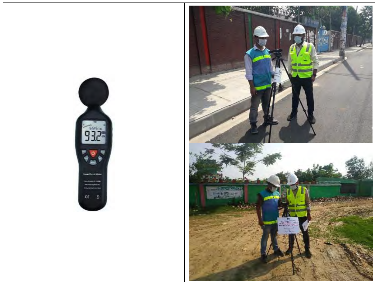
Figure 4-23: Ambient Noise Level Monitoring equipment (Tekcoplus)
