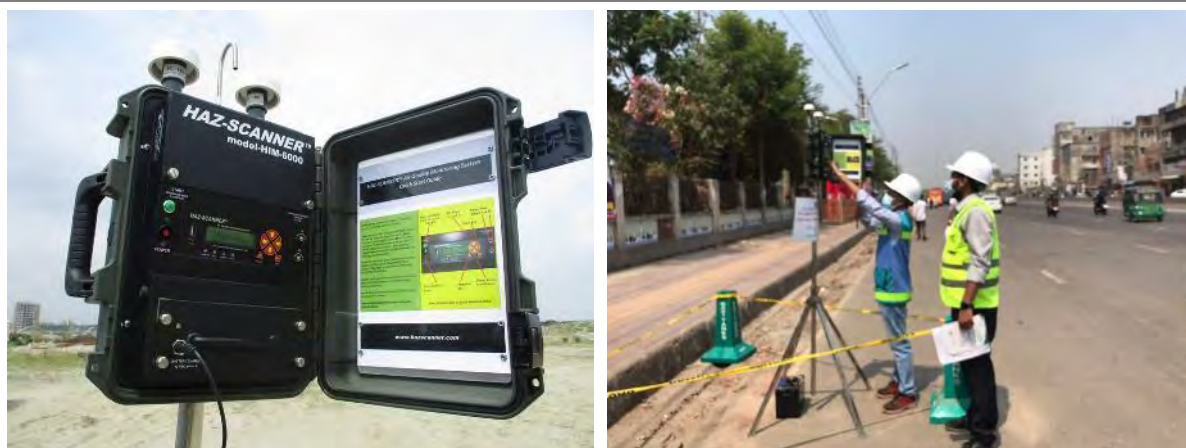
Figure 4-20: Ambient Air Quality Monitoring Equipment (Haz Scanner: HIM 6000)
