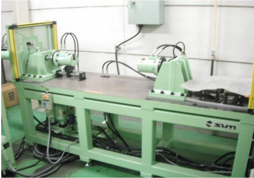
Oil Damper Test Equipment
