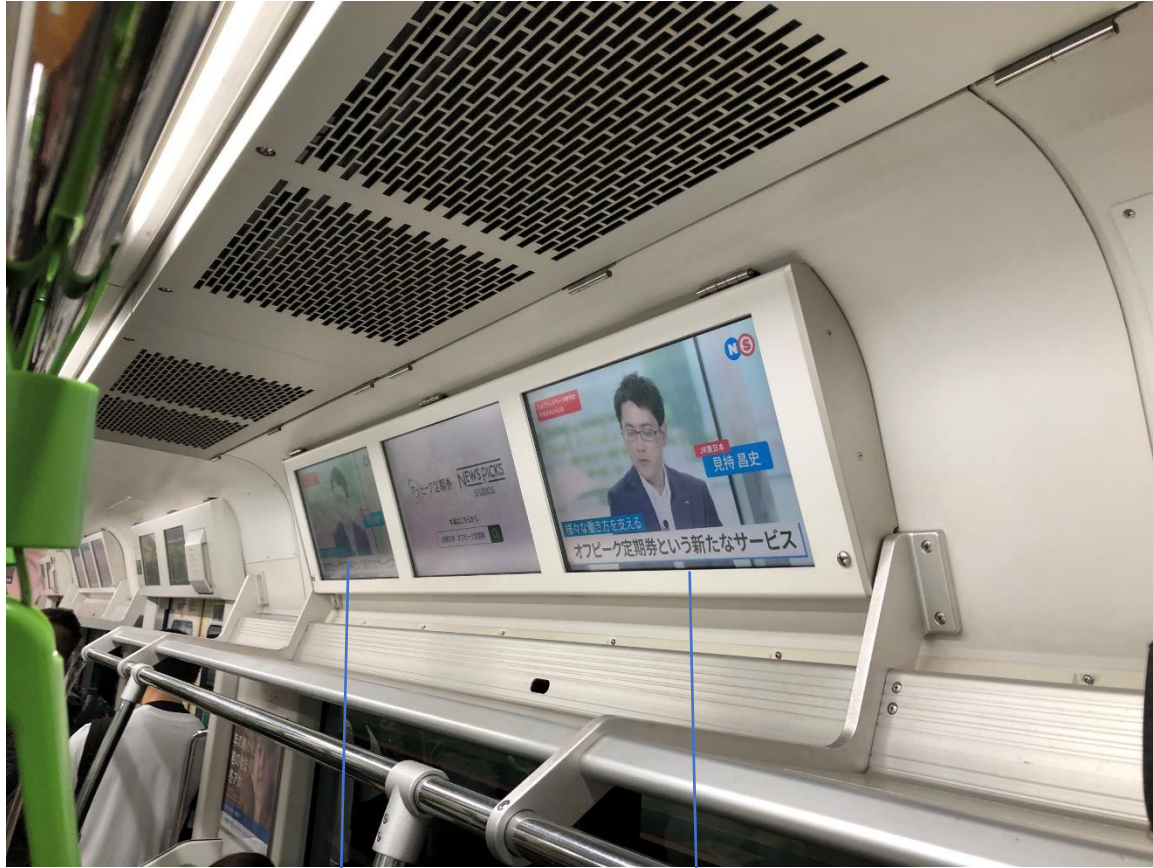
Three (3) Extra LSD (LCD saloon Display) for advertisement content just above the fixed window
