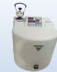
Planetary Ball Mill, FRITSCH, Pulverisette 6
