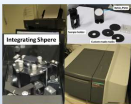
UV-VIS-NIR Spectrophotometer, Shimadzu 2600
