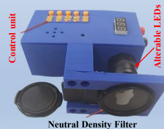
Light Source with Variable Wavelength, Intensity and Illumination Period
