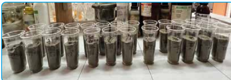
Fig.: Image of release test of CRFs in soil
