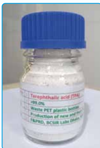
Terephthalic acid (TPA) monomer from waste PET plastic
