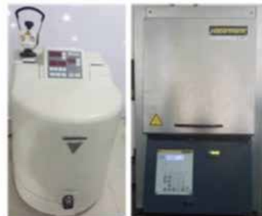
Planetary Ball Mill(Left) Programmable HT Furnace(Right)
