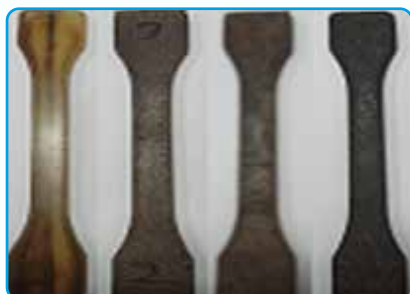
Injection molded PO-Jute composites
