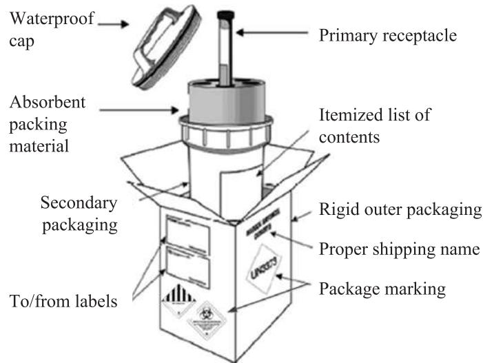
Figure 6.1 Triple package for transport of infectious specimen
