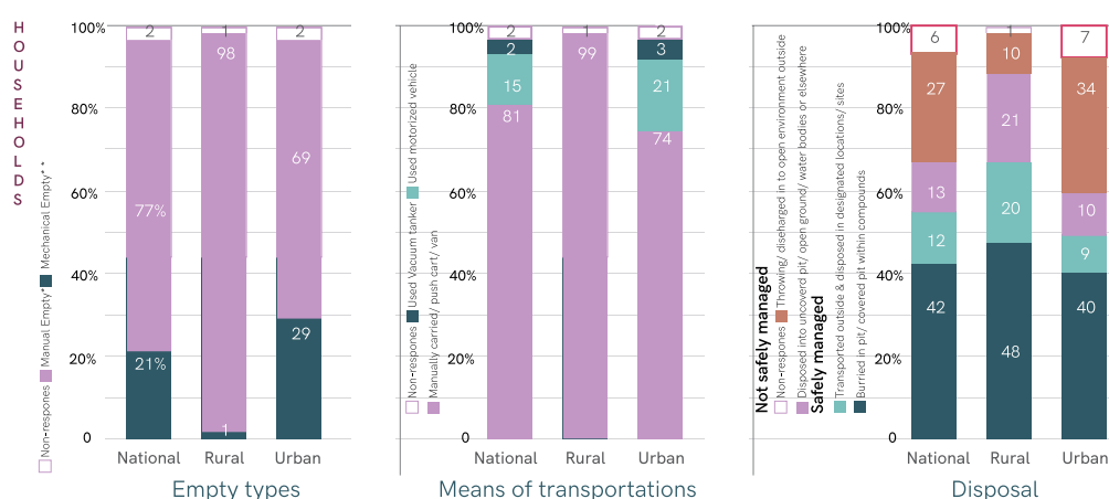
Figure-10: Emptying, transportation and disposal of fecal sludge from HHs improved on-site facilities with adequate containment
