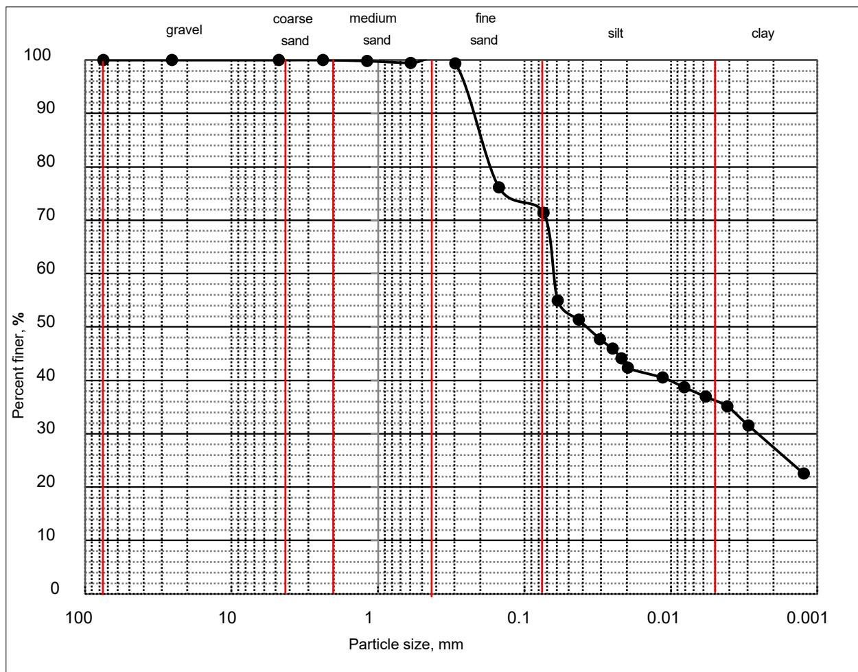
**PARTICLE SIZE ANALYSIS OF SOILS BY SIEVE & HYDROMETER**
