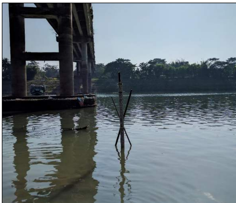
Figure 6-1 Installed Water Level Gauge on the Surma near Sylhet Bypass Bridge (Station ID: S-06)
