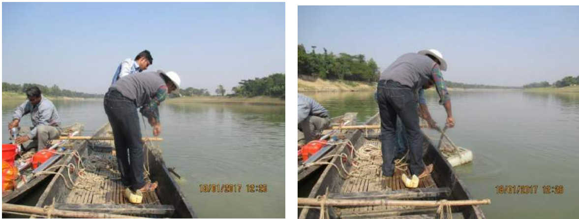
Figure 6-2 Collection of Sediment Concentration Samples
