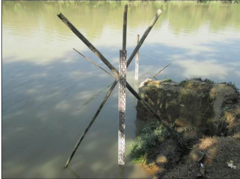
Figure 6-8 Installed Water Level Gauge on the Kushiyara near Sherpur Bridge (Station ID: K-03)
