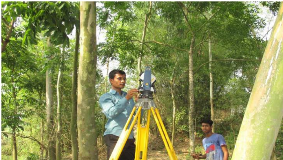
Figure 3: Riverbank Survey by Electronic Total Station
