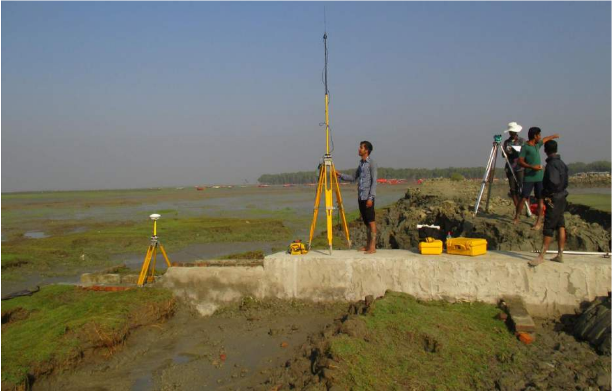
Figure 2: Establishment of Coordinates With RTK GPS
