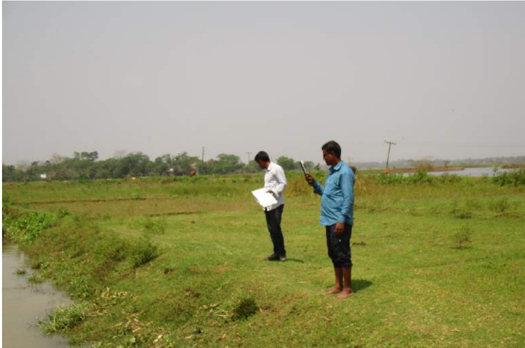
Figure 6: Establishing a Point by RTK GPS
