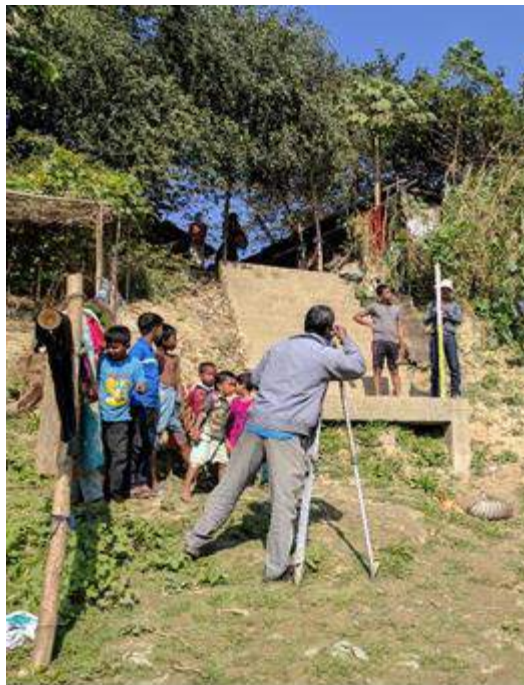
Figure 7: Riverbank Survey by Electronic Total Station
