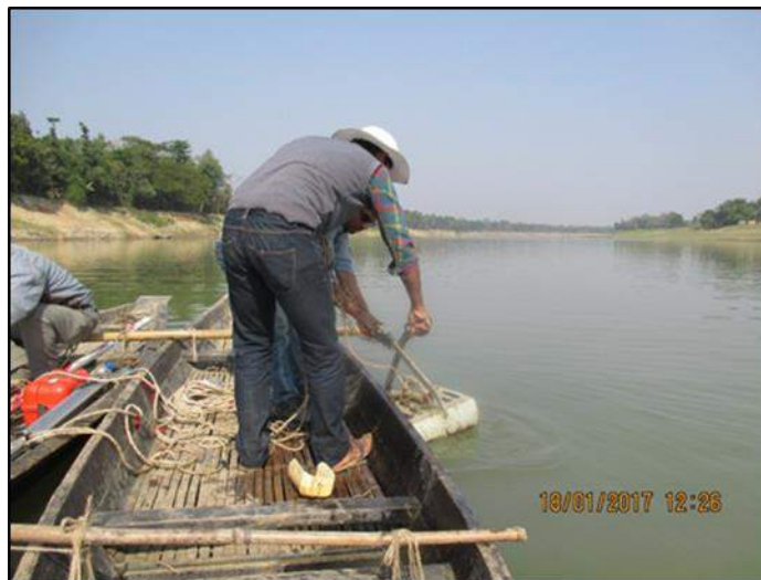
Figure 6 Surveyors collecting bed material samples using the sampler
