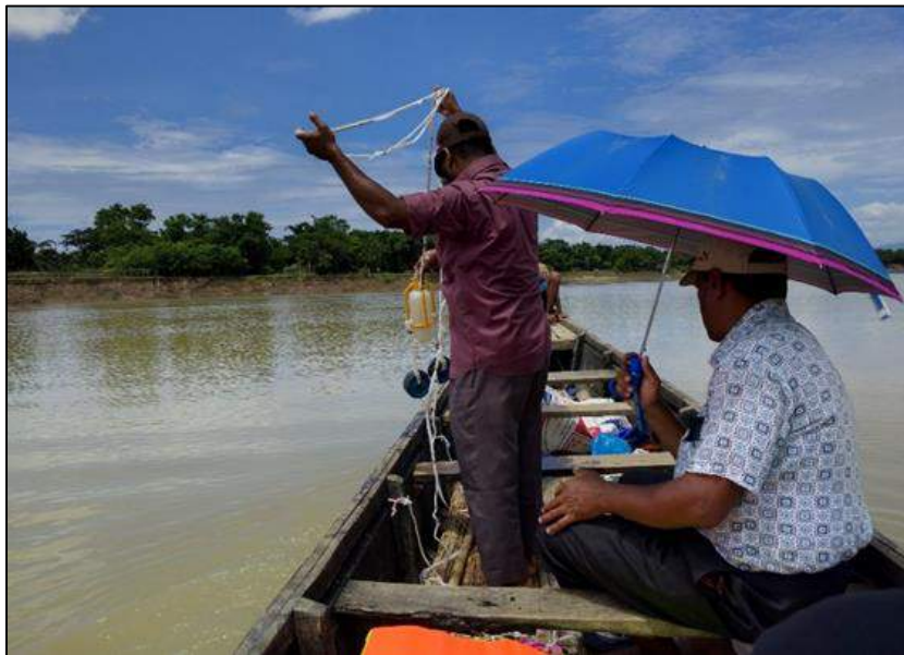
Figure 1 Sample collection bottle is being lowered by ropes
