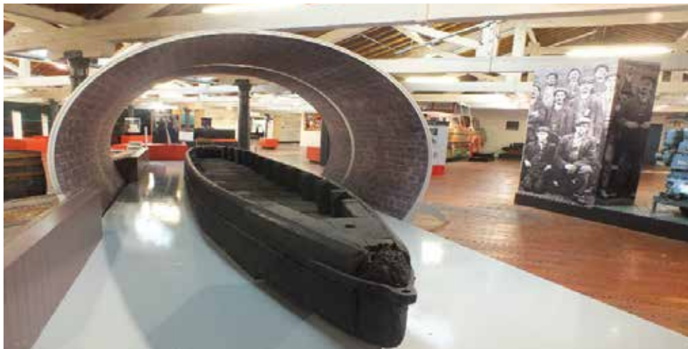
James Brindley designed a box boat named Starvationer with 10 wooden containers in 1766
