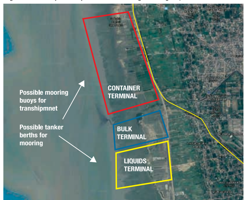
Figure-7: Overall Layout of Bay Terminal to Meet Cargo Handling Requirements
