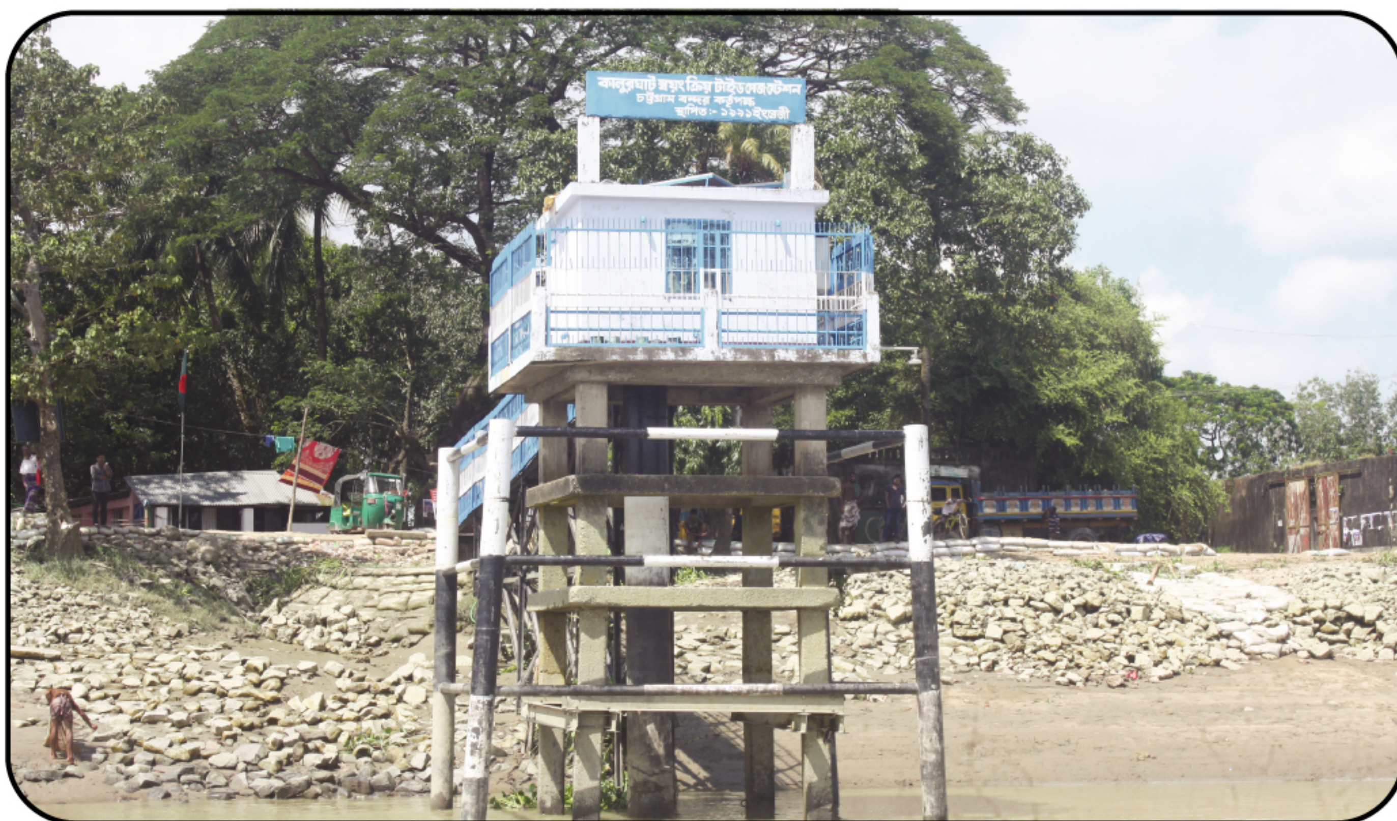
Auto Tide Gauge Station at Kalurghat
