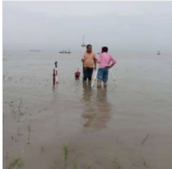
Plate 4-1: Photograph of Bay Terminal Water Level Measurement
