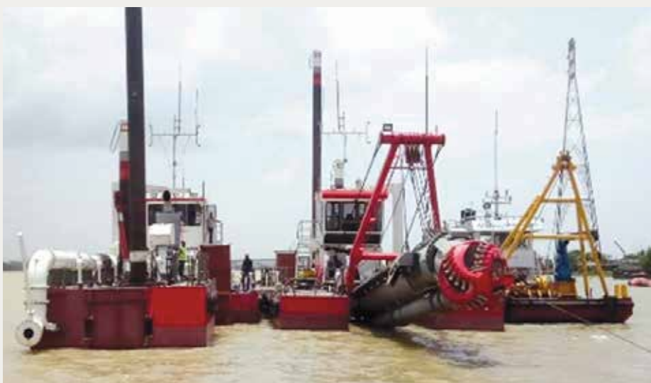
This type of dredger is used by the Chittagong Port Authority to maintain the navigability of the Karnaphuli river.
