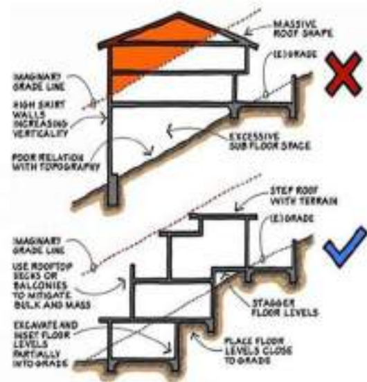
Figure 12-3: Construction Strategy on Hillside.
