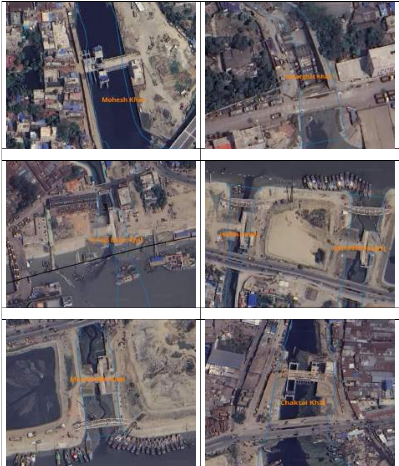
Figure 3.4. Width Constriction at Khal Outlets by Regulators
