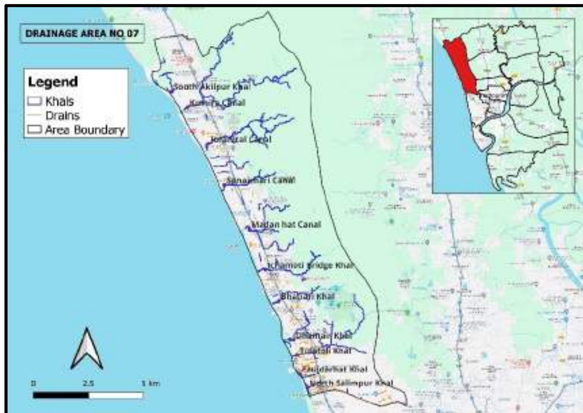
Figure A1-7 Drainage Area No. 07
