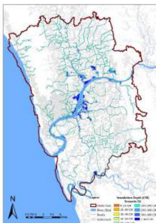
Figure 5.5b: Flood inundation due to spring tide (Scenario 02)
