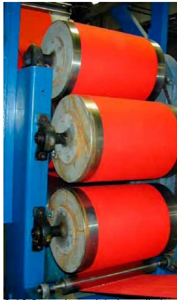
2.12 Steam heated drying cylinders.
