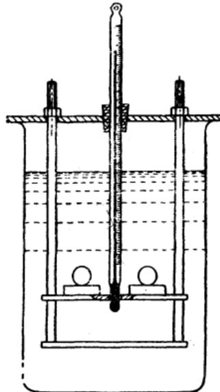
Fig. 1 Assembly of Apparatus for Determination of Softening Point (Ring and Ball - Two Rings)
