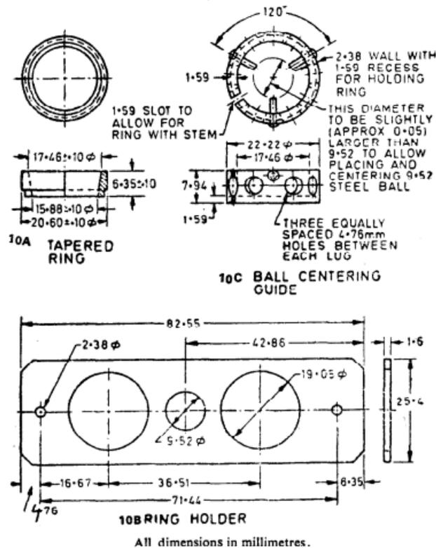
Fig. 2 Components of Ring and Ball Apparatus
