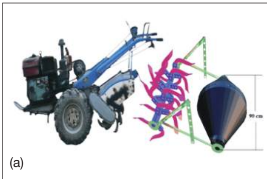
Fig1. Pictorial view of (a) Earthing Up Machine and (b) field operation
