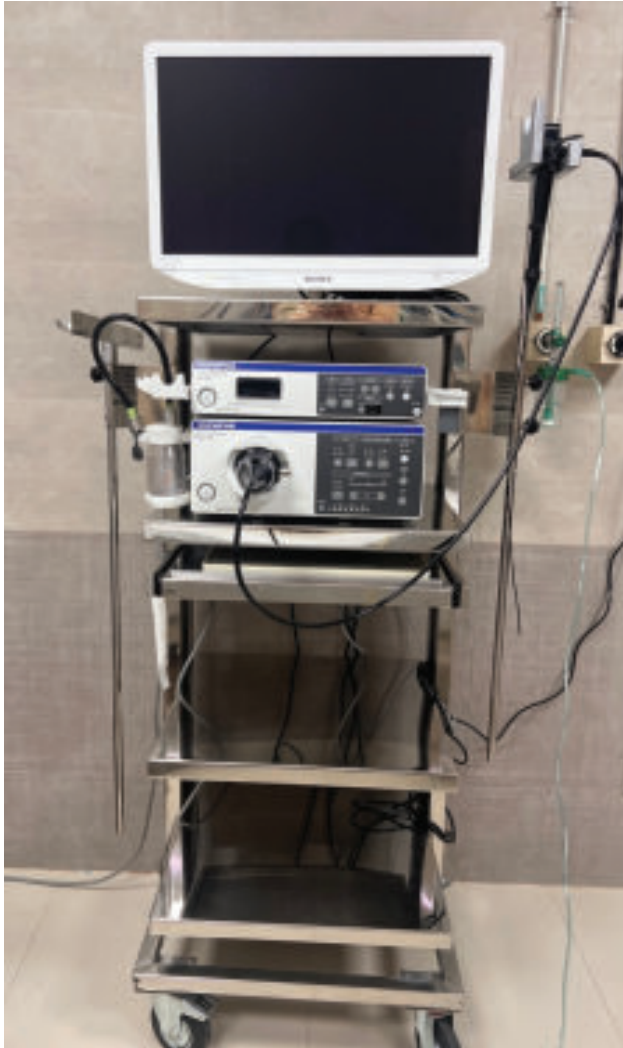
Fig.-3 Portable cart having video processor, video monitor & video recording system and bronchoscope
