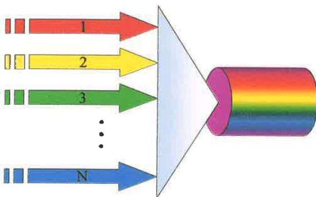
A separate light wavelength carries each signal and the dense in DWDM refers to its ability to accommodate different wavelengths.
