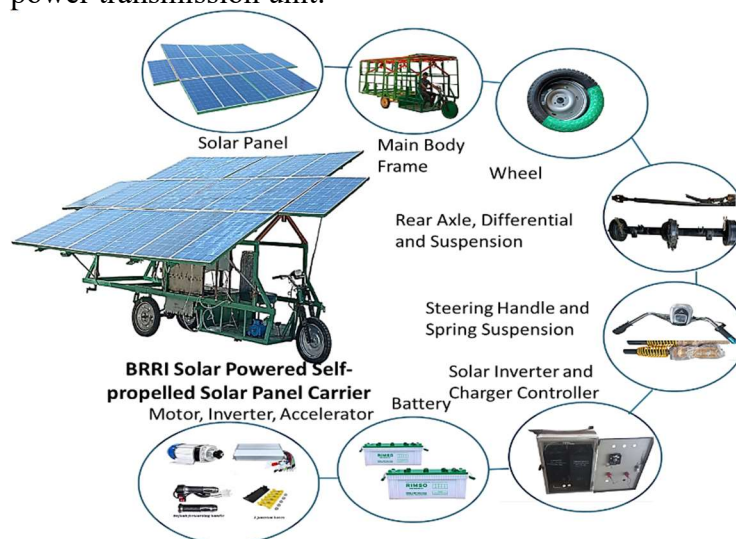
Fig. 11. Overview of the developed solar power system
