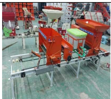
Plate 2. BRRI Automatic Seed Sower Machine in operation
