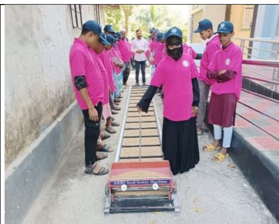
Plate 27 (b) Operation of manual seed sower machine
