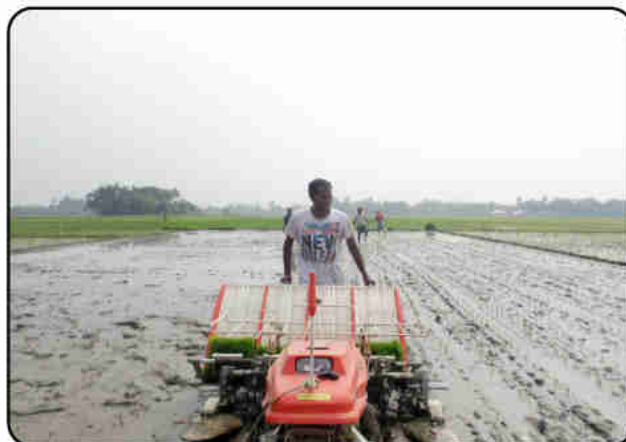
Photo 3.7: Transplanting operation using mechanical transplanter
