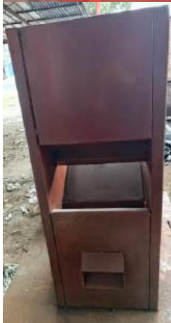
Main Body: The main frame and body are made with a 1.8 mm MS sheet. The length: 600 mm, width: 495 mm, height: 1125 mm.
