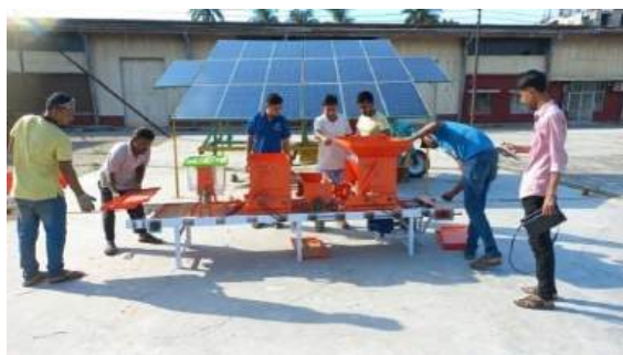
Plate 6a. Solar-powered BRRi auto seed sower machine.
