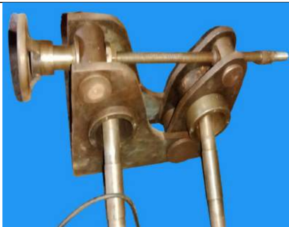
Roller attachment. This parts attachment included the tyeter, roller shaft, bearing block
