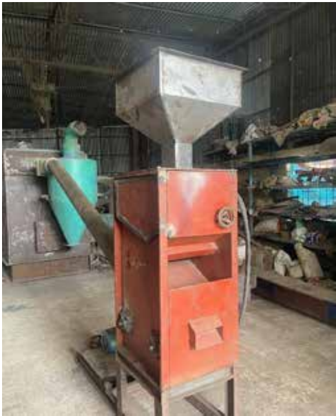
Fig 8. Pictorial view of de-husker
