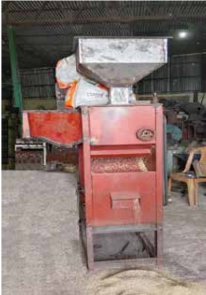
Fig 9. Operating condition of de-husker
