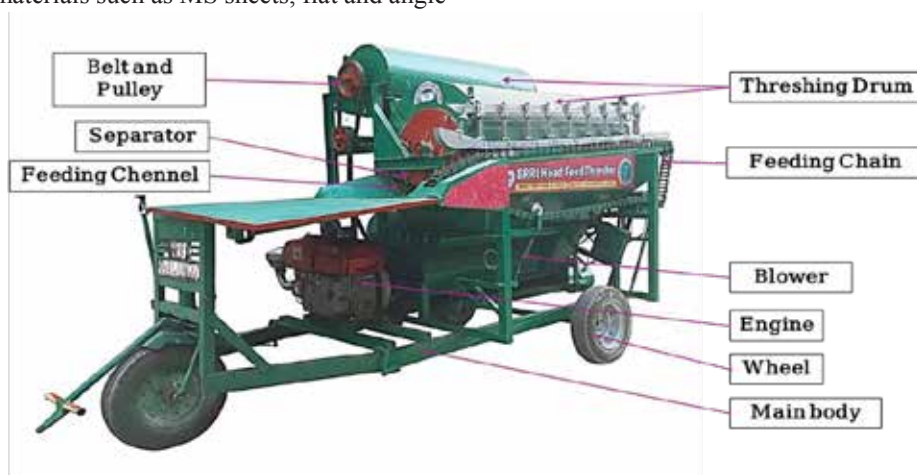
Fig. 6. Head Feed Thresher and its functional parts
