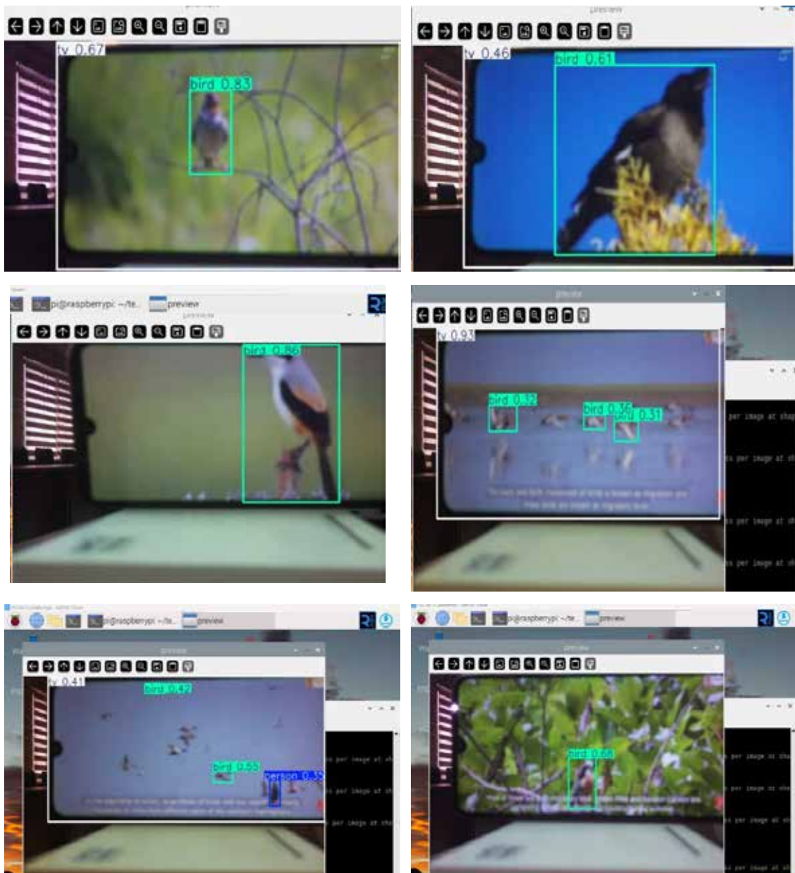
Fig. 2. Real-time bird detection results using YOLOv8n on a Raspberry Pi 4. Each image shows the bounding box and confidence score for detected birds.
