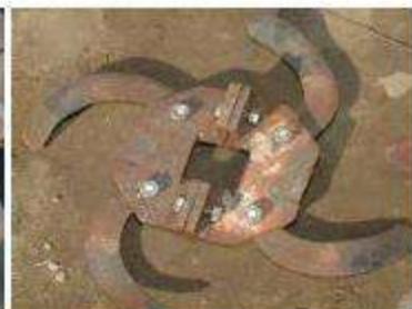
Photo 9 Tyne holder with bracket
