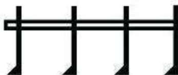
Fig. 2 Tyne arrangement of planter in ST mode
