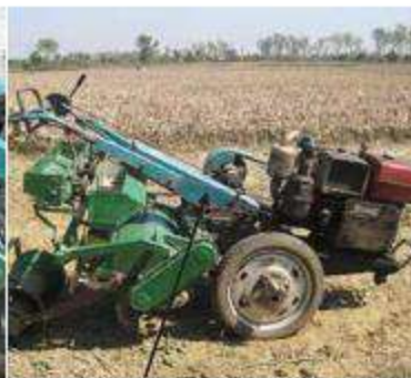
Photo 7 VMP attached without extra gear box
