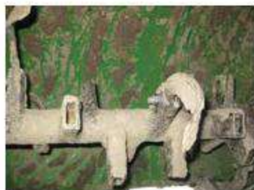
Photo 3 Round rotary shaft with fixed tyne holder
