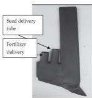
Photo 10 Seed and fertilizer delivery line
