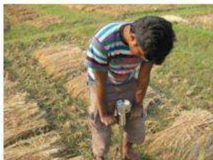
Photo 1 Measurement of soil penetration resistance
