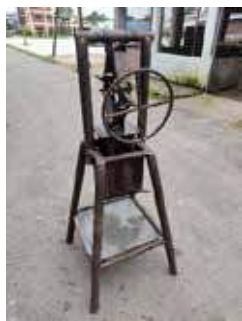
12a. Fabricated prototype of the manually operated briquette machine
