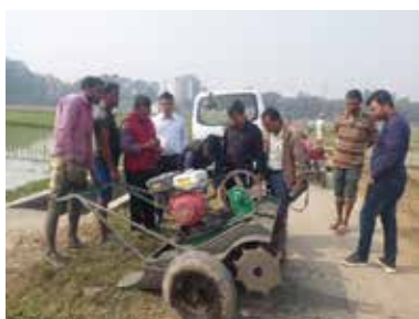
Plate 6. Test of modified hydro-tiller at BRR West Byde, Gazipur.
