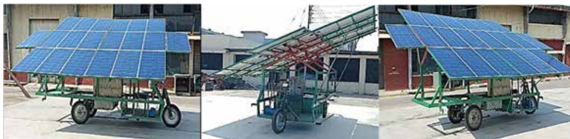
Plate 17. Solar-powered self-propelled mobile solar panel carrier
