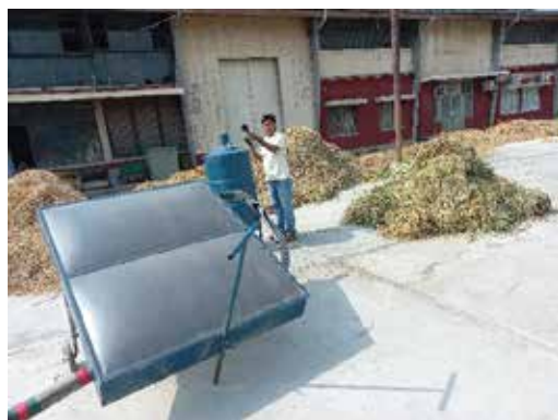
Plate 16. Performance test of the developed dryer
