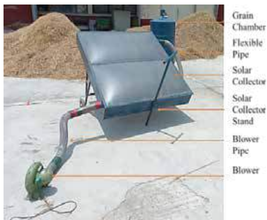
Plate 15. Complete view of the developed dryer
