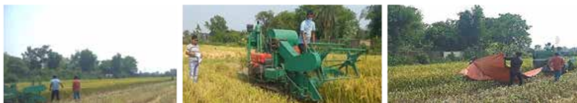
Plate 2. Performance test of the developed whole feed combine harvester.
