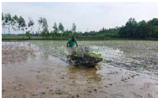
Plate 7. BRRI developed rice transplanter cum mixed fertilizer applicator.
