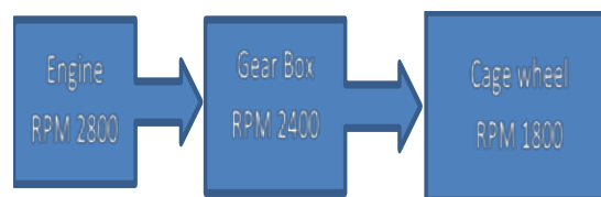
Fig. 6. Flow sheet diagram of power transmission system of the modified hydro-tiller.
