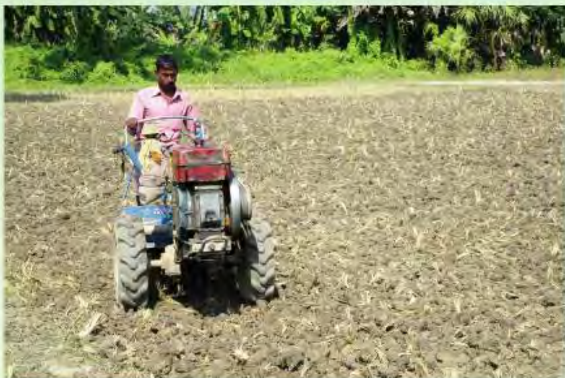
Photo 3.3 Tillage by power tiller
