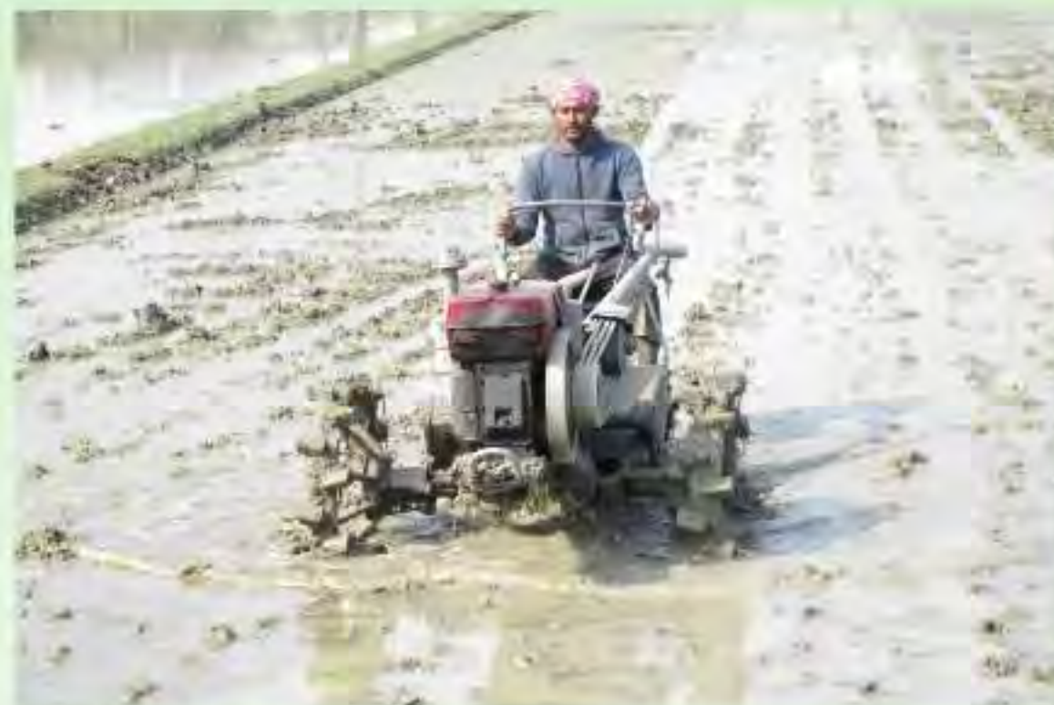
Photo 3.3 Tillage by power tiller
