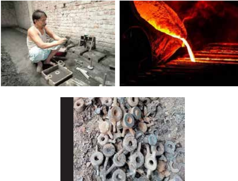
Fig. 11 : Mold making, molted alloy pouring and casted unfinished parts
