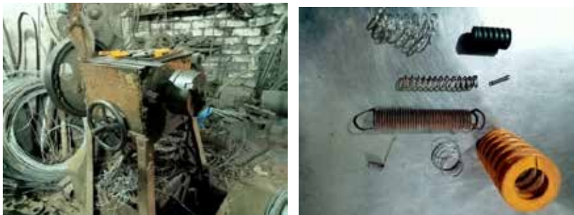
Fig. 26 : Coiling machine (special type of lathe) and manufactured springs
