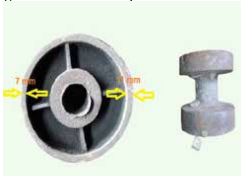
Fig. 11: Pattern failure of track roller
