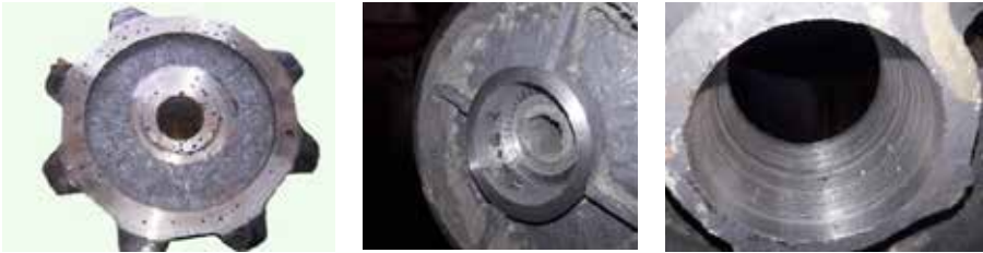
Fig. 12: Porosity developed in sprocket and track roller for improper casting design
