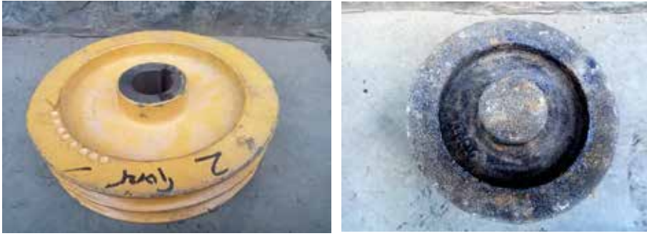
Fig. 13: Fan belt pulley and its excess metal pouring when casting
