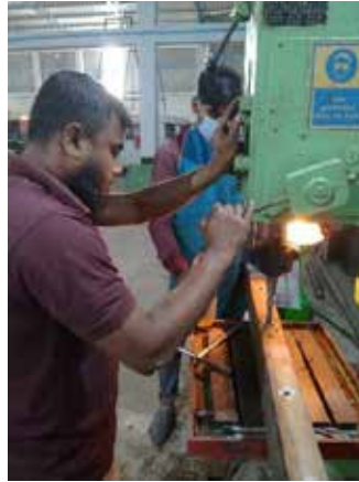
Fig. 15: Drilling of harvester chassis.
