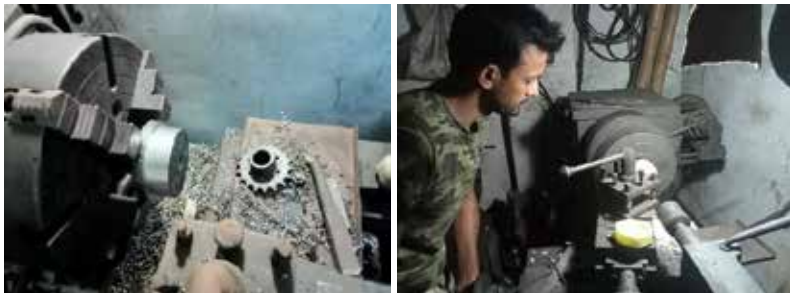
Fig. 13: Machining of driving chain wheel and fuel tank cap in lathe machine
