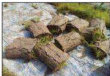
Photo 28 Mat damage by rodents and excessive soil height
