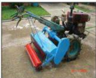
Photo 5 BARI high speed rotary tiller
