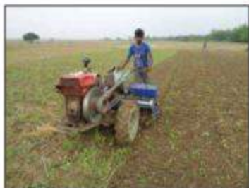
Photo 4 Power tiller operated seeder (PTOS) for seeding jute seed
