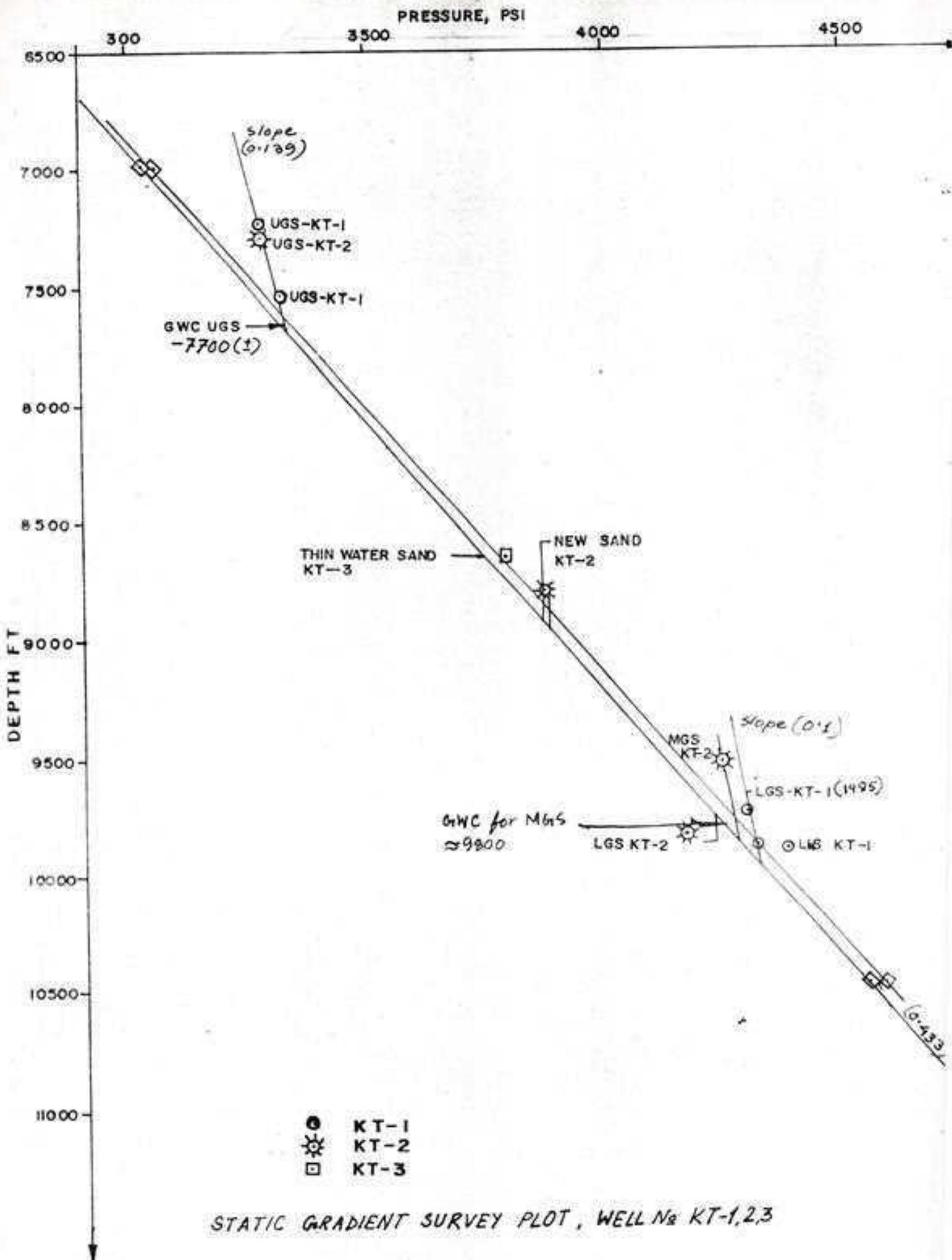
STATIC GRADIENT SURVEY PLOT, WELLS KT-1,2,3
